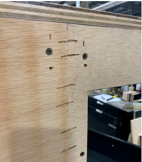
Corrugated staples ensure tight panel joinery.
